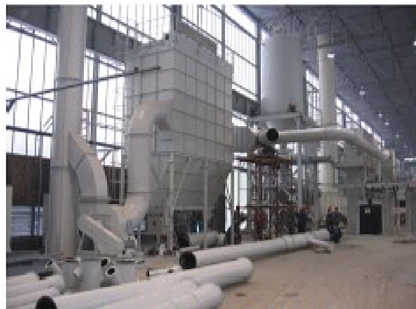
Dust collector IKV 4,0-240-387 Capacity 35.000 m 3 /h
