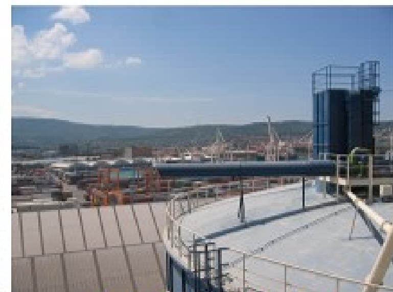
Dust collector FVS 3,0-144-176 Capacity 15.000 m 3 /h
