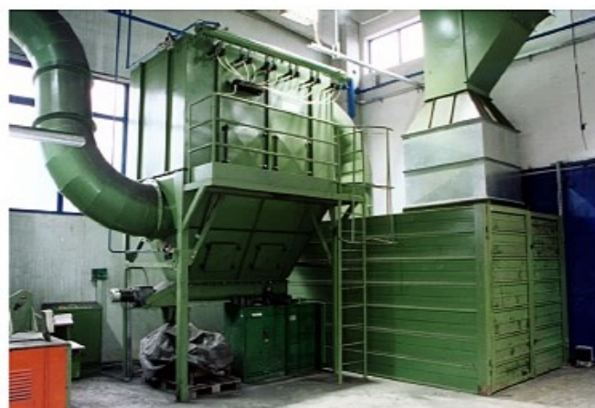
Cartridge Dust collector PF-24 Capacity 25.000 m 3 /h
