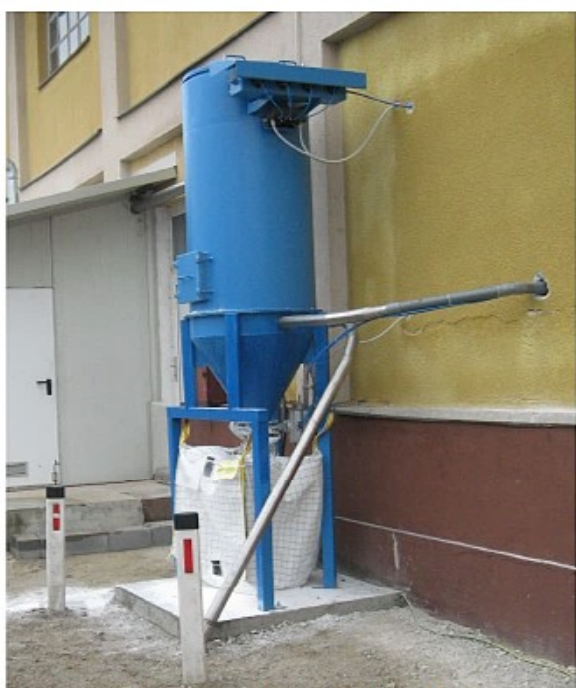
Vacuum cleaner VC-400 Capacity 400 m 3 /h
