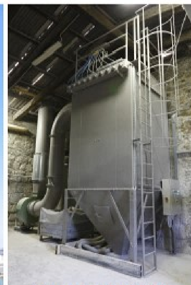
Dust collector FVL 2,4-100-98 Capacity 10.000 m 3 /h
