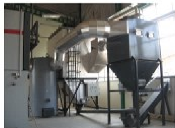
Dust collector IKV 3,0-160-196-PT Capacity 10.000 m 3 /h (200 °C)
